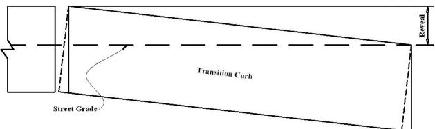
All transitions longer than 6.9' will be manufactured in the field by the setter from standard curbing.
