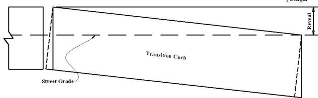
All transitions longer than 6.9' will be manufactured in the field by the setter from standard curbing.
